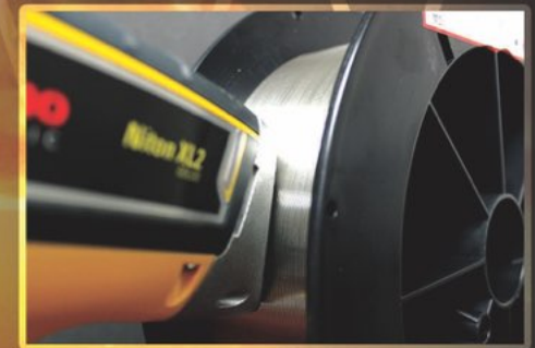
All incoming raw materials are 100% verified with XRF for compliance to specifications
